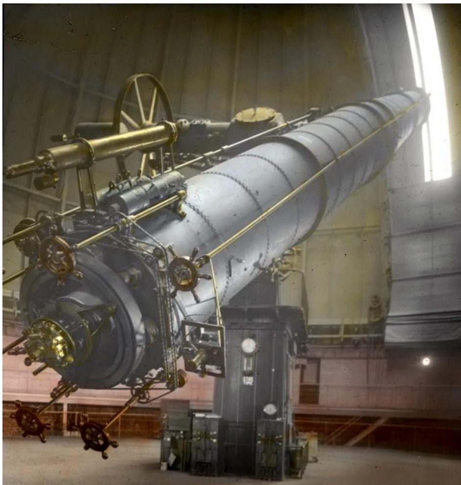
Figure 3. The 101.6 cm «Clark» refractor, with a focal length of 19,4 m, of the Yerkes Observatory, in Wisconsin, USA (Ferreri 1989, pp. 199 and 202). Still the largest refractor in the world in operation today.
